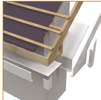
Standard over fascia installation
